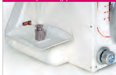
Calibration of the balance
